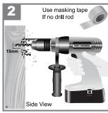
Drill your holes with a 10mm drill bit making sure not to drill more than 15mm deep by using a drill depth rod or the masking tape wrapped around the drill bit back from the tip of the drill bit.
